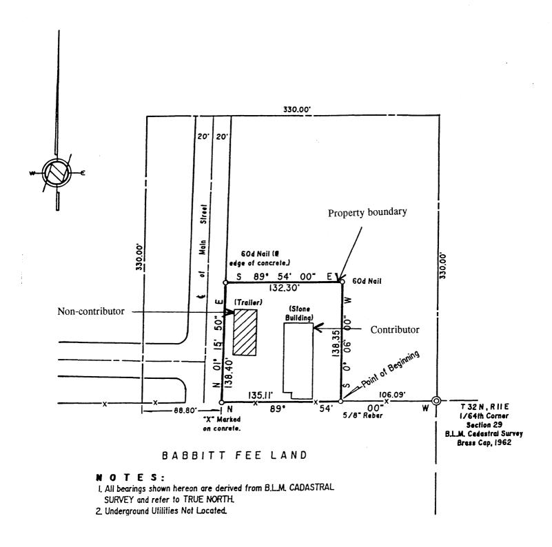
Figure 2. Boundary of the Krenz-Kerley Trading Post property, showing contributing building (historic trading post) and non-contributing building (modern trailer).
