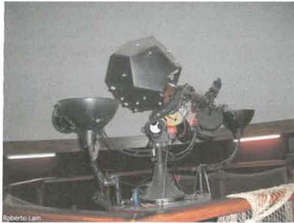
Figure 5. The picture shows the Spitz A2 Projector, full-dome, installed for the Fountain of Youth Planetarium. (Photograph: Lam, Roberto. Accessed April, 2015. http://www.aplf-planetariums.info/en/index.php?onglet=planetariums&menu=sheet_planetarium&filtre=1408 .)
