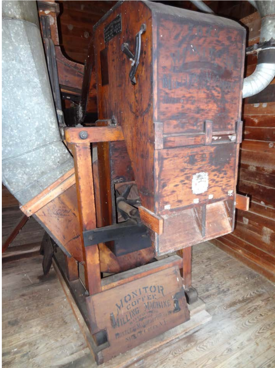
Figure 5: Second floor of the mill, Monitor Milling Machine, built by Huntley Manufacturing Company to clean coffee beans, but used to clear shelled corn at Dillard Mill, photograph, January 2014, from the files of the Missouri State Historic Preservation Office.
