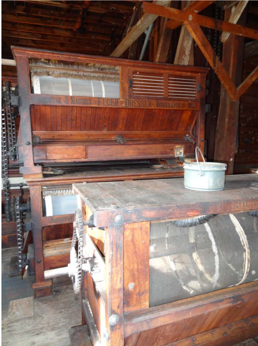
Figure 6: Second floor of the mill, flour dresser (sifter) built by Nordyke and Marmon, originally covered with silk screens, but restored in 2005 with nylon screens. In front of this is the Barnard and Leas Reel sifter used to sift corn meal. January 2014, from the files of the Missouri State Historic Preservation Office.
