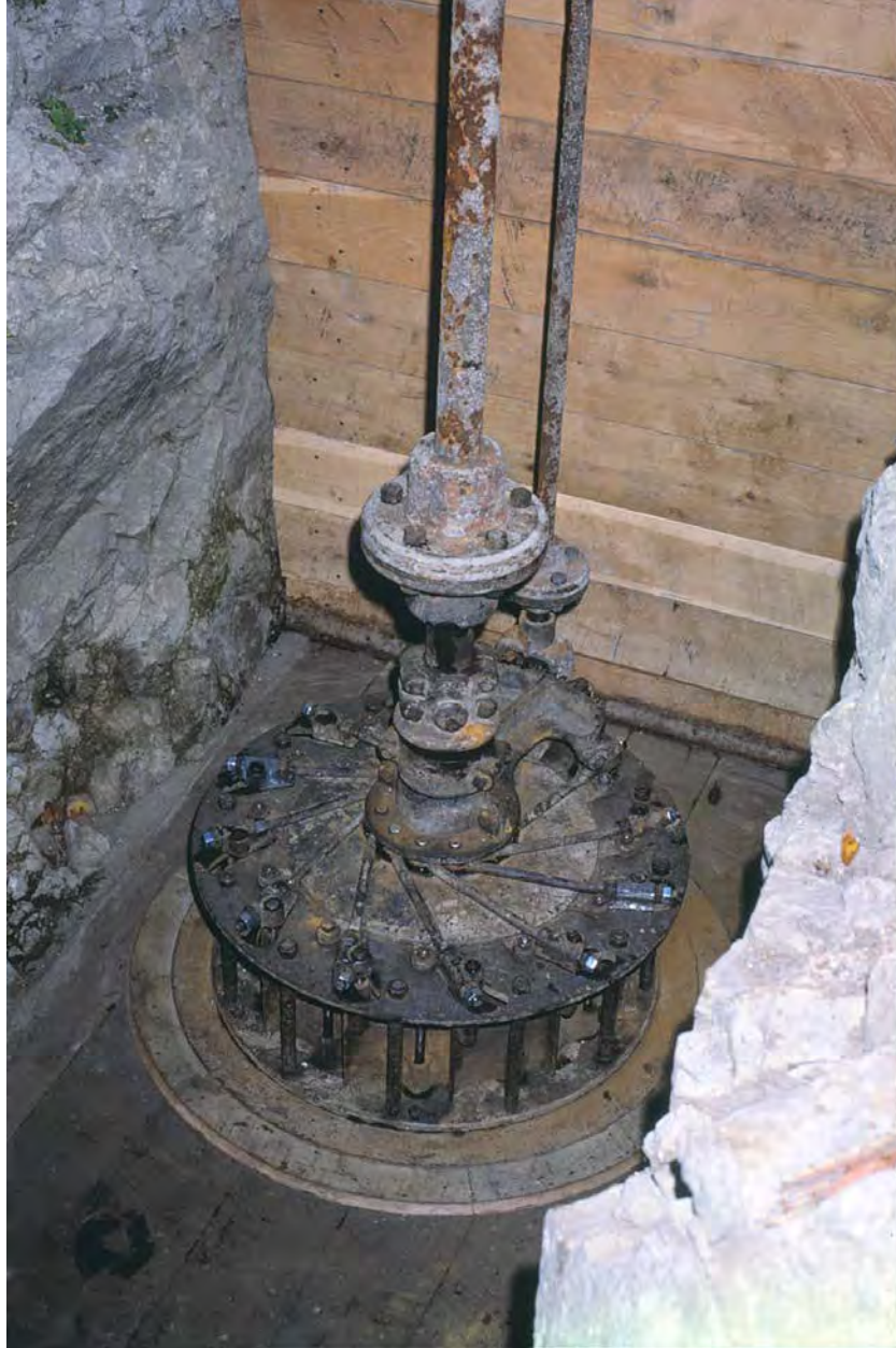
Figure 2: Turbine at Dillard Mill, photographed by Derek Ogden during restoration project (1928).
