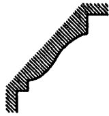
CROWN MOLDING AT SECOND FLOOR 12" x 1 1/2" x 1/2" 11
