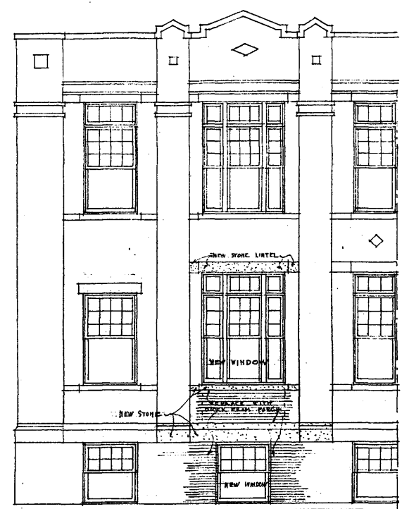
REVISED ELEVATION WITH ENTRANCE REMOVED AND WITH 2nd FL. AND BASEMENT WINDOWS SHOWN PATCH ALL FINISHED WALL WHERE ORIGINAL WORK SHOWS DAMAGE REPEAT THIS ELEVATION OPPOSITE END.
