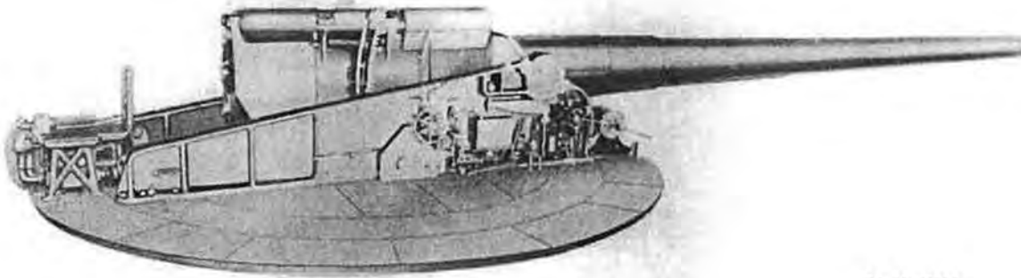
Figure 1—Gun, 16-in., Mk. II, M1, Navy, and Carriage, Barbette, 16-in., M4 — Right Side View
