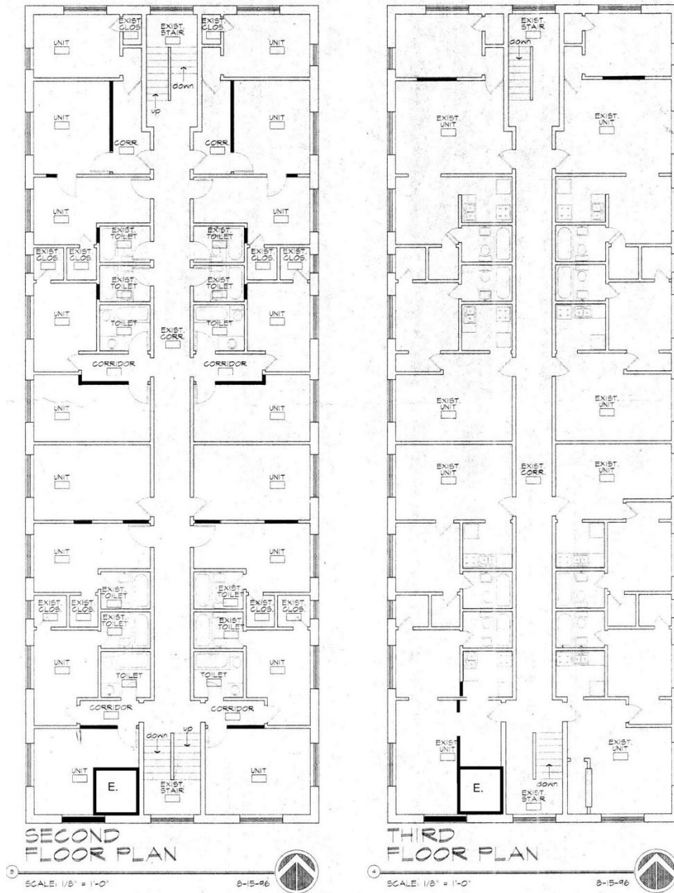
Figure 6. Floor Plans, Second and Third Floors. Darkened walls indicate 1990s changes. Base plans courtesy of nomination sponsor Jason Murray.
