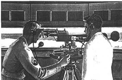
Figure 5: Howard S. Schroeder, a commercial artist in New York, spent three years as a mine planter with Battery B of the 21st Coast Artillery at Fort Miles. This 1943 painting shows how the fire control towers of Fort Miles worked: two men armed the azimuth and were connected to the plotting room via the headsets visible here. The window sash behind the men are the same as the upper observation slit window of Tower No. 23. 5
