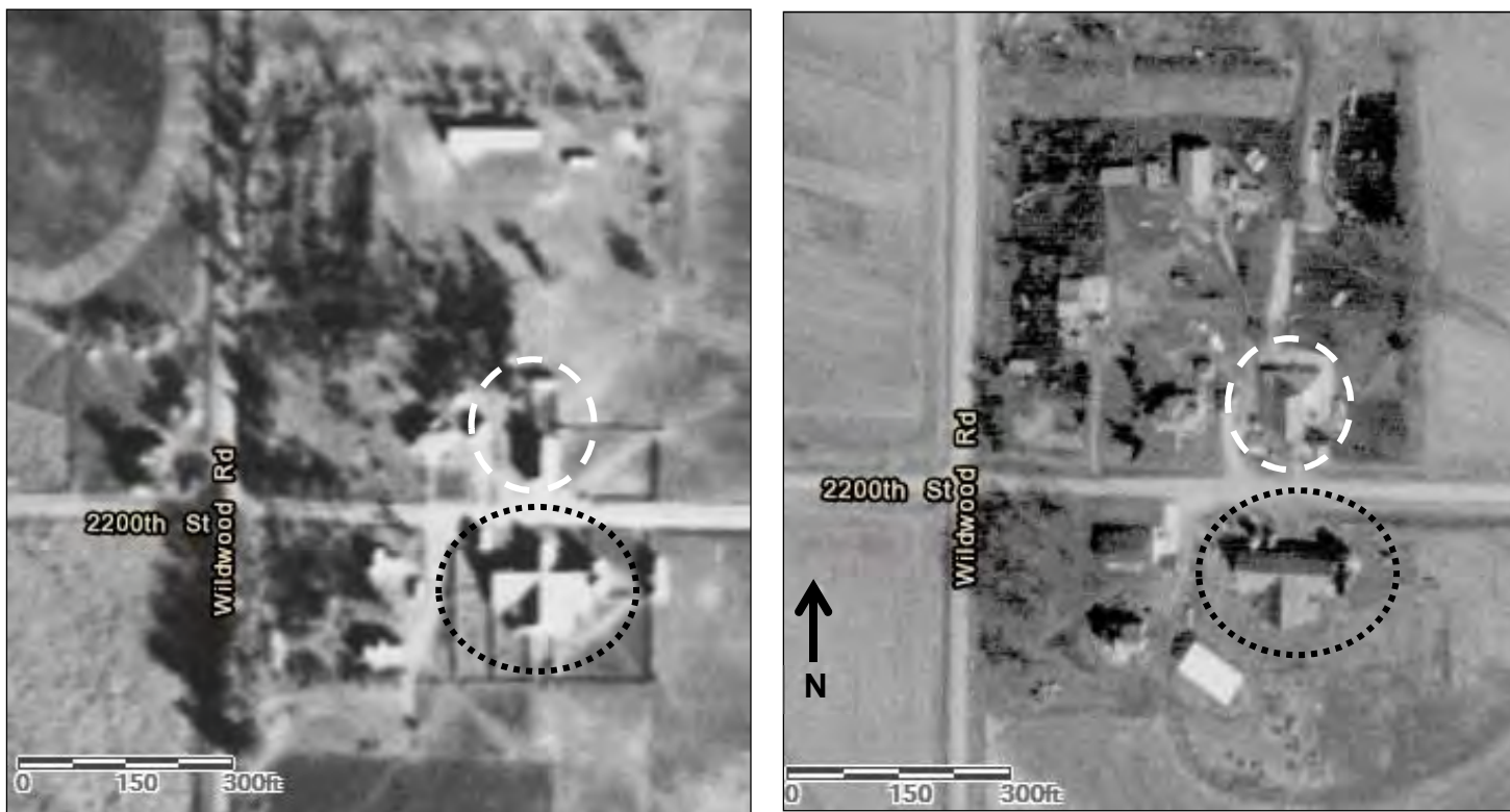
Figure 62. A late 1930s aerial photograph (left) and a 1990s aerial photograph (right) show the location of the cross-shaped barn (black dotted circle) and the front-gabled transverse-frame barn (white dashed circle) at Escher's Long Branch Farm. Note that by the 1990s, the cross-shape of the barn had been altered to a T-shape and a large wrap-around shed had been added to the front-gabled barn. The cross-shaped barn was destroyed by fire circa 2010 and later replaced by a modern shed; the front-gabled barn is extant. Source: Iowa Geographic Map Server, 2018.
