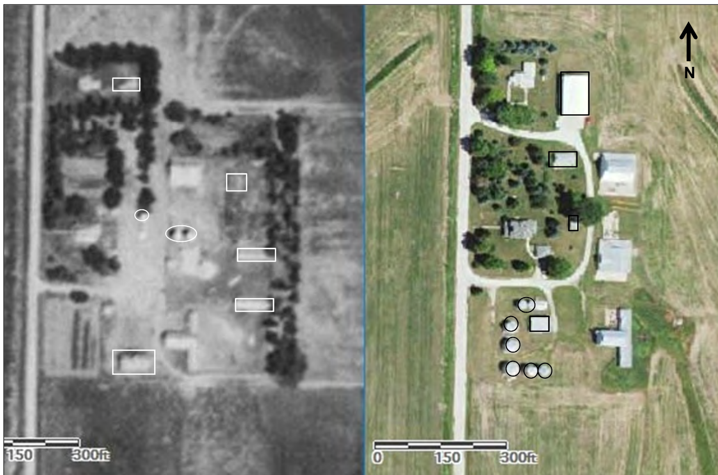
Figure 47. Left: Late 1930s aerial photograph with buildings and structures that appear to have been removed outlined in white. Right: 2017 aerial photograph with buildings that have been added since the 1930s outlined in black. Maps obtained from the Iowa Geographic Map Server 2018.
