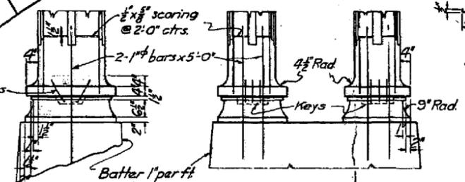
DETAILS OF PEDESTALS Scale 1/2" = 1'-0"
