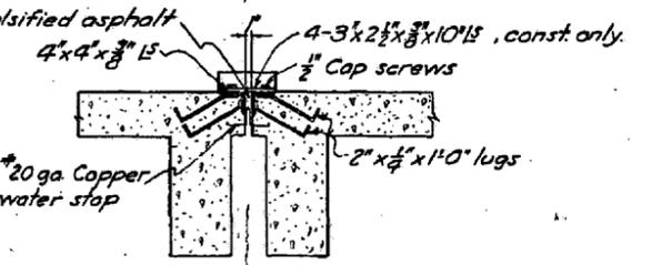
EXPANSION ANGLES at points 0-11 & 23 of each span
