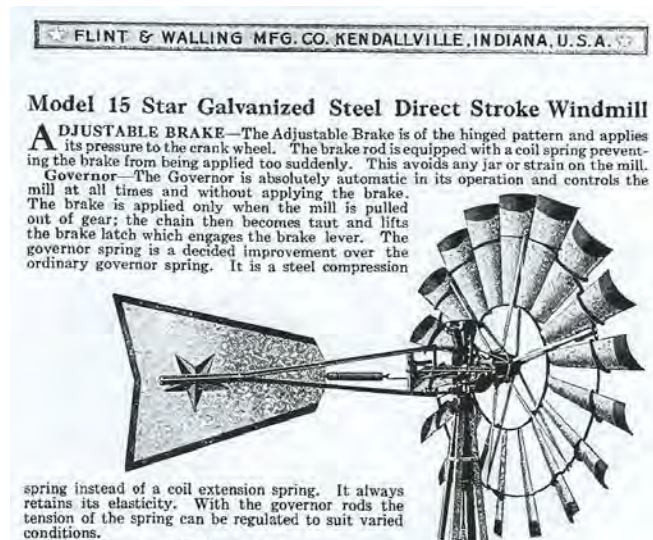
Figure 23 Flint & Walling Mfg. Co., Star Windmill Catalog , 1920 Model 12 and 15 windmills
