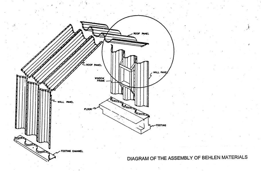
Diagram shows how side and roof members are joined by bolted connections to form continuous self-supporting arch.
