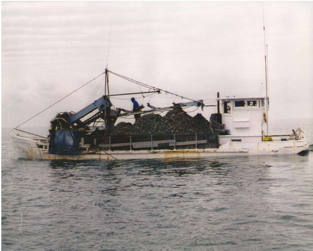
Historic Photograph #16: CASHIER , dredging under power, 1980s. Note conveyor belts and machinery on deck and square stern.
