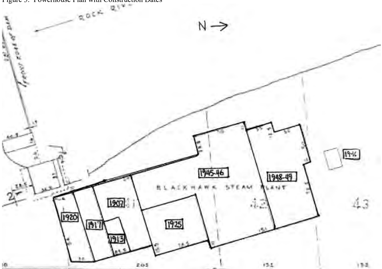
Figure 3. Powerhouse Plan with Construction Dates
