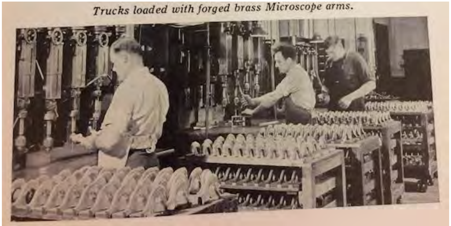
Figure 11: Forging machines used to shape microscope stands.
