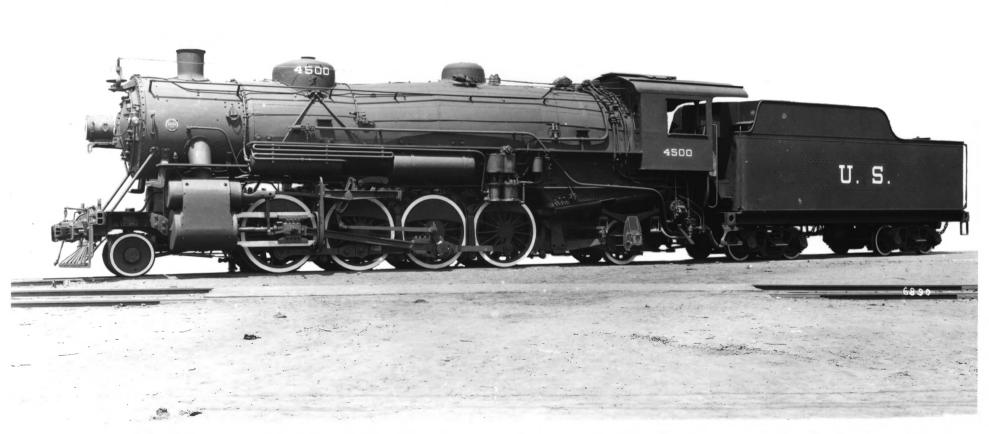
Baltimore and Ohio Railroad steam locomotive No. 4500 . . . the first USRA light Mikado locomotive, identical to Lake Erie & Western 5541/ Nickel Plate Road 587 when built. "U.S." on tender flanks denotes USRA control of B&O and other major railroads. 1918-1920.
