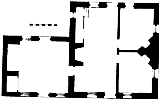
The Quaker Plan in the Valley of Virginia Fairfax Grant Farm. The Quaker plan of the central block with an added wing room.
