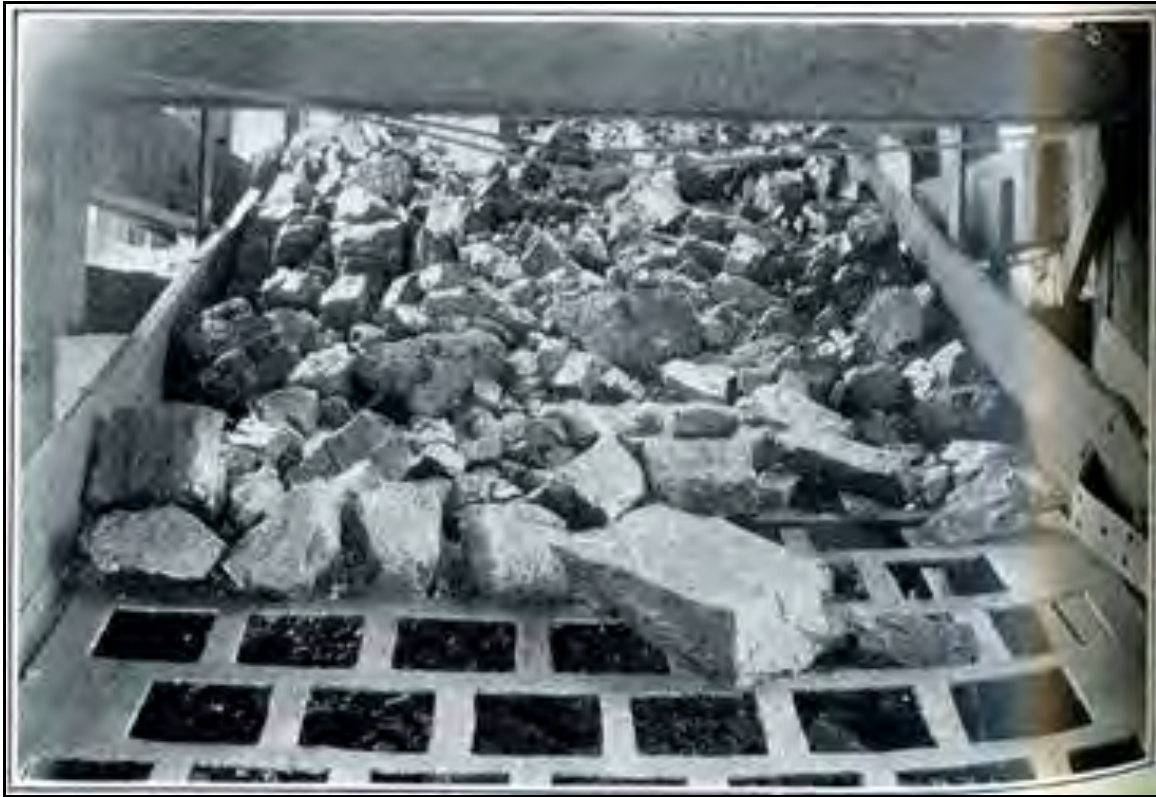
Figure 9: Lump coal screen, Ravenscroft tippel, Tennessee Products Corporation. Photo courtesy of The Southern Tennessee Coal Field by Wilbur Armistead Nelson.
