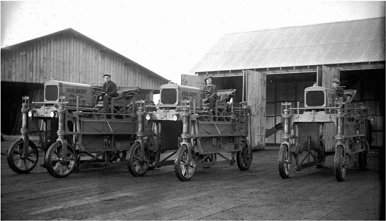
Three Ross Straddle Lumber Carriers at the Hulbert Mill. c.1915. Photo courtesy of Jones Historical Photo Collection
