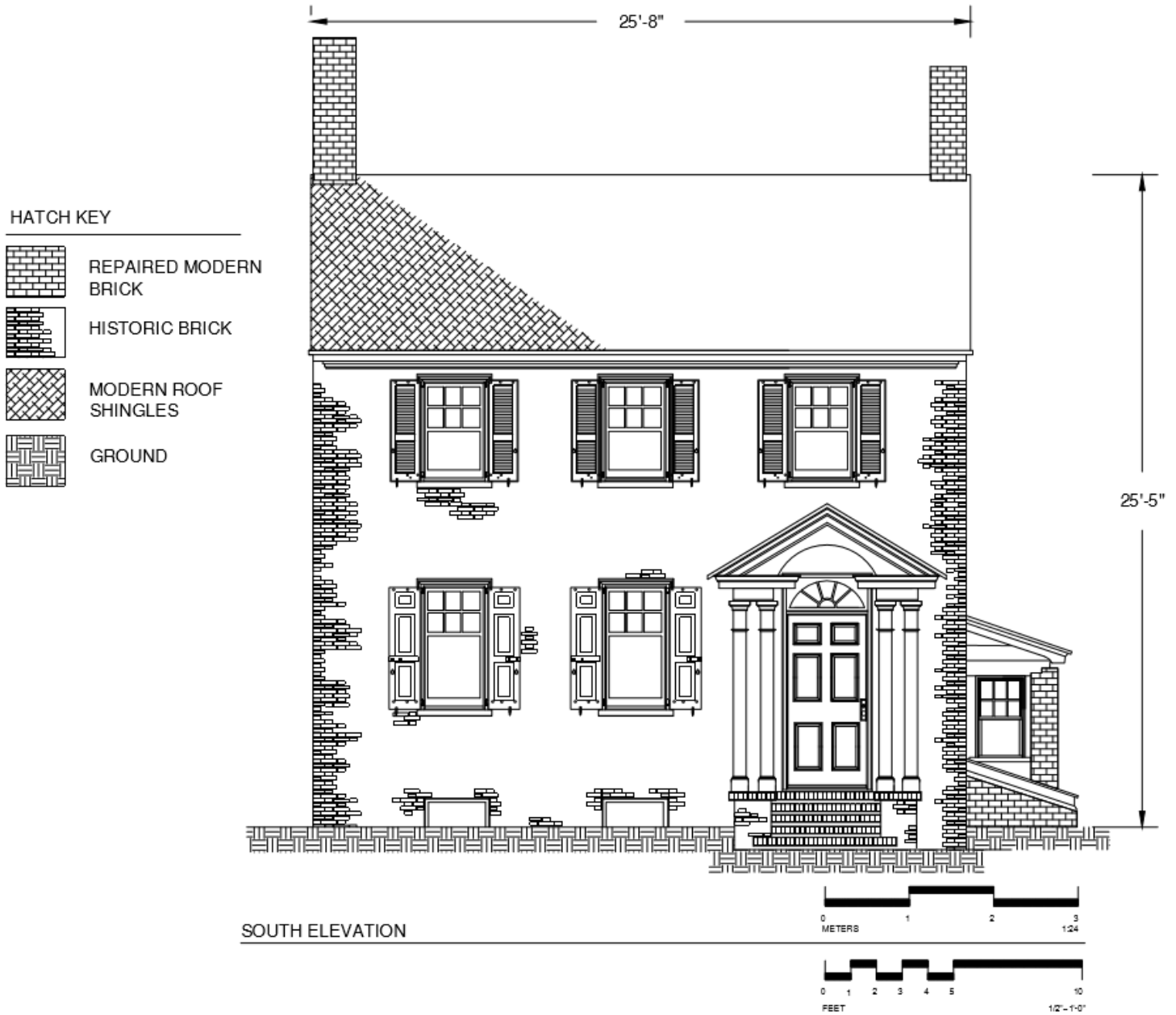
Figure 4: Drawing of the south elevation of the Elkinton-Butcher House, 9564 Highland Street. (Drawn by: Virginia Davidowski)
