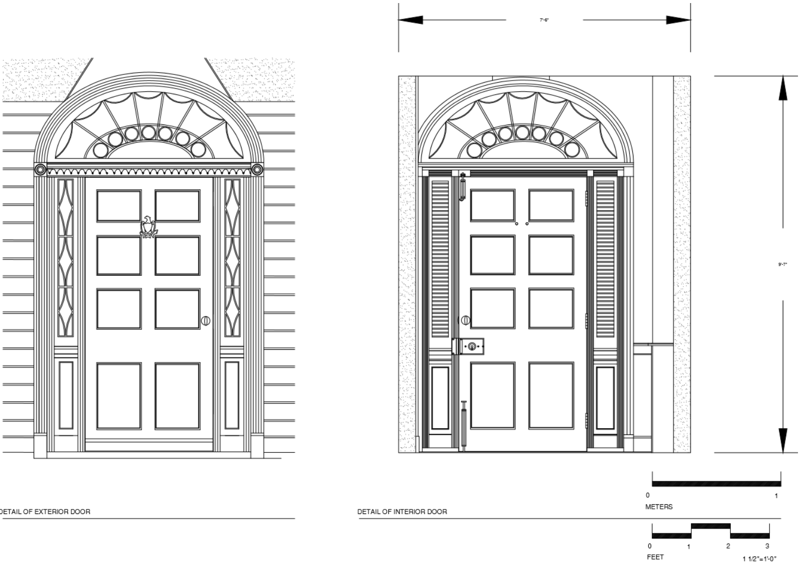
Figure 6: Detail drawings of the front door (exterior and interior views) of the Captain David Compton House, 1201 Front Street (Drawn by: Michael J. Emmons, Jr.)
