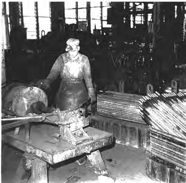
■ Figure 23. Cliff Stewart bending and threading brake beam rods in Roundhouse, circa 1960.
