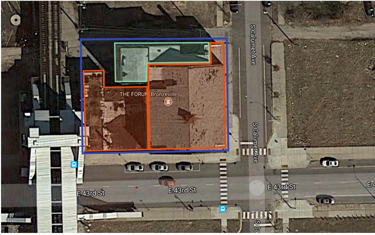
FIGURE 2: SITE MAP OF THE FORUM HALL. *Note property boundaries (blue), original 1897 construction (orange), and historic 1900 addition (green).
