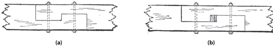
Figure 4.38 (a) Straight tabled scarf joint, (b) with key. From Jacoby, Structural Details , 126
