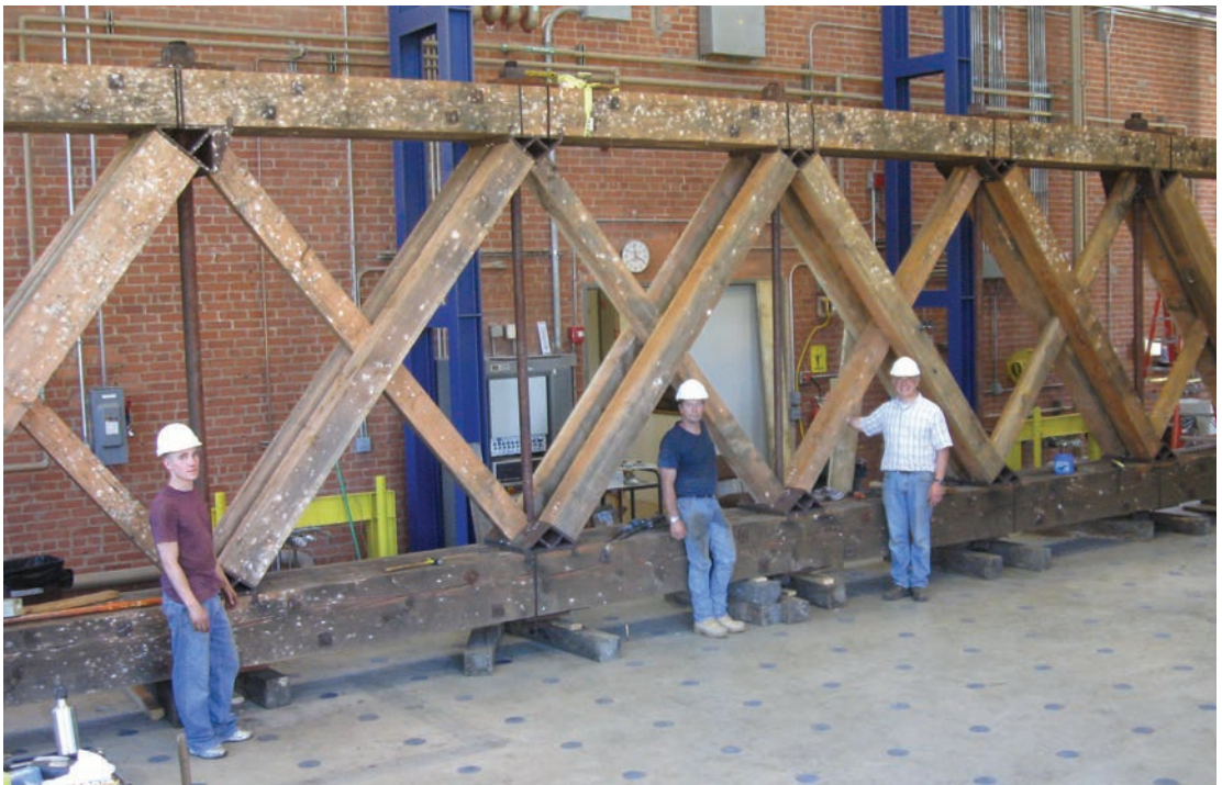
Figure 2.5 FHWA funded a joint project between HAER, Case Western Reserve University, and the National Society for the Preservation of Covered Bridges to study the Moose Brook Bridge (1918) in Gorham, New Hampshire, a Howe truss that was a victim of arson in 2004. The original castings were restored, and bridgwright Tim Andrews reconstructed the salvaged trusses for testing in Case Western’s lab. Top 2.5a) The burned trusses sat idle for five years. HAER NH-48-3, Jet Lowe, photographer, 2009. Above 2.5b) The first truss assembled in the lab. Photograph courtesy Dario Gasparini, 2011.
