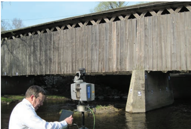
Figure 2.3 New technologies for documentation include HAER's Leica C10 scanner and the FARO scanner used by the University of Minnesota–Duluth. Top Left: 2.3a) A Leica C10 scanner was used to document the West Union Bridge (HAER IN-105). Jeremy Mauro, photographer, 2013. Top Right: 2.3b) Resulting point cloud of West Union Bridge. Scan data by Jeremy Mauro, 2013. Left: 2.3c) A FARO scanner was used to document the Cedarburg Covered Bridge in Wisconsin. Brian K. Brashaw, photographer, 2010.
