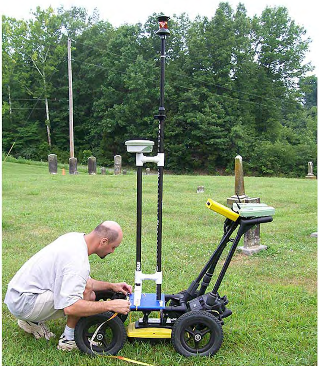
The Noggin Smart Cart ground-penetrating radar (GPR) system configured with 500 MHz antennae, a GPS antenna, and a total station prism. Camp Ground Cemetery is in the western background.
