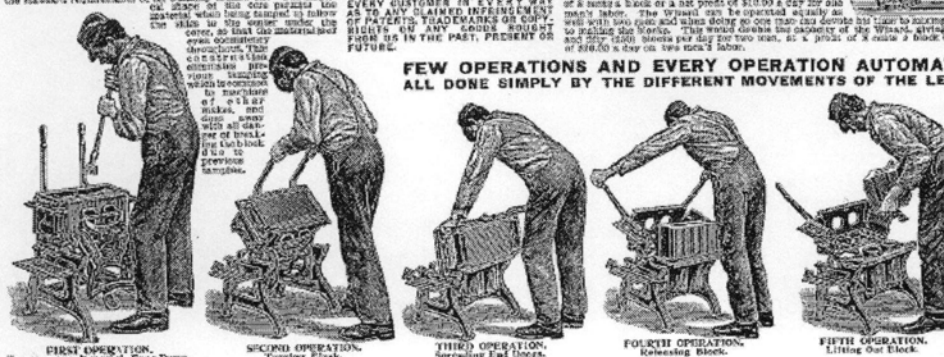
FIRST OPERATION. Tamping the material, Face Down. SECOND OPERATION. Turning the Face Lever. THIRD OPERATION. Spreading the material. FOURTH OPERATION. Releasing the block. FIFTH OPERATION. Lifting the block.
