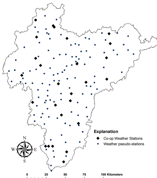
Figure 10. Weather stations in the high-density cooperative network used to generate daily values for each of the pseudo-stations in the SWAT model.
