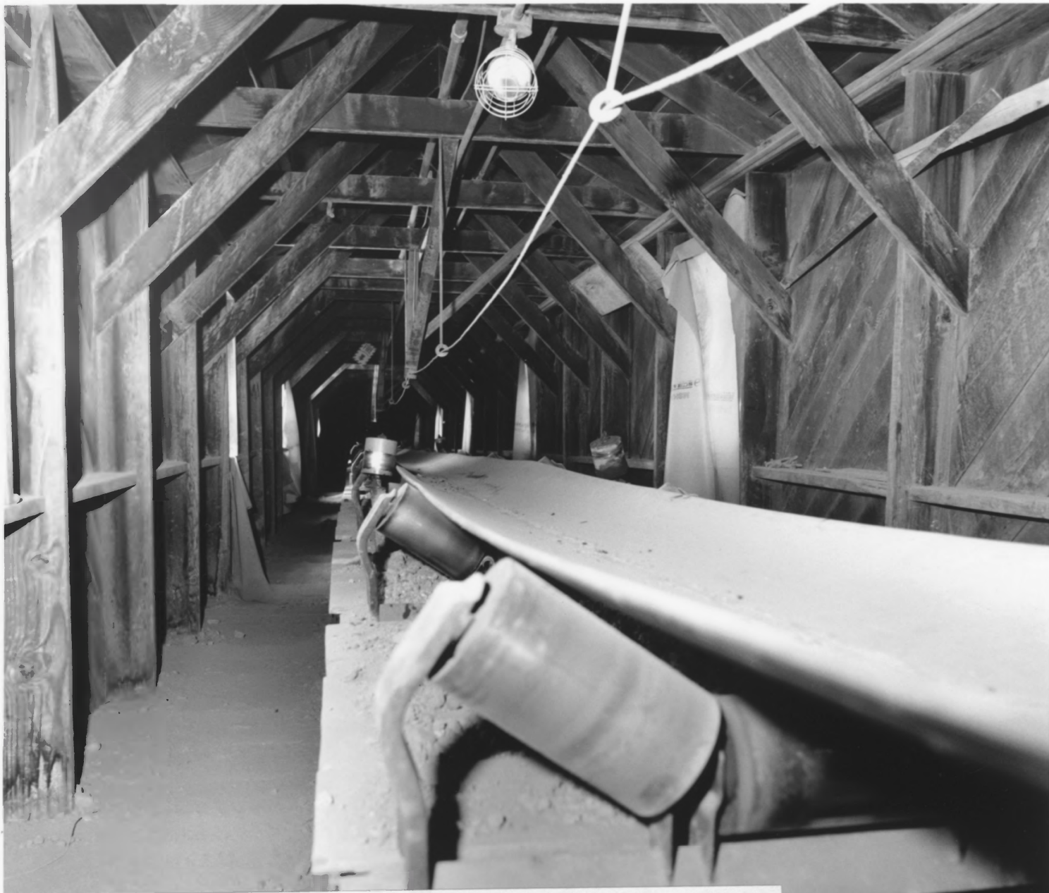
Photograph #22 Shenandoah-Dives Mill Silverton Vicinity, San Juan County, Colorado Interior of 200 ft. Conveyor with Belt (#1 on Flow Chart) Frederick Athearn, Historian, San Juan County Historical Society, September 1995
