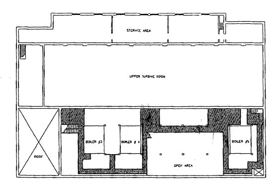
Figure 3. Third floor plan, Fremont Municipal Power Plant and Pumping Station.
