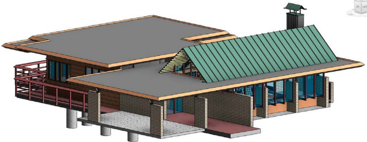
Figure K. Front view of house with covered carport in the foreground, and standing seam copper roof over living room. Revit model by Thomas Rex Hardy, AIA.
