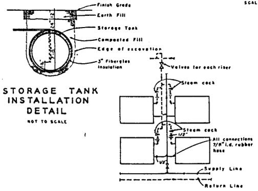
**STORAGE TANK INSTALLATION DETAIL**
