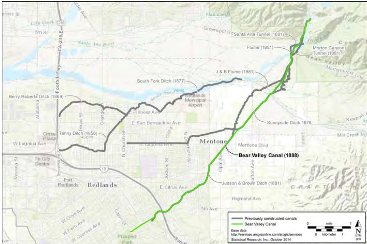
Figure 19 Time Series 1889 Map - Upper portion of Judson and Brown Ditch abandoned and Sunnyside improved under the Bear Valley Water Company. Upper portion of Sunnyside and lower portion of Judson and Brown together from the Redlands Canal/Bear Valley Canal.
