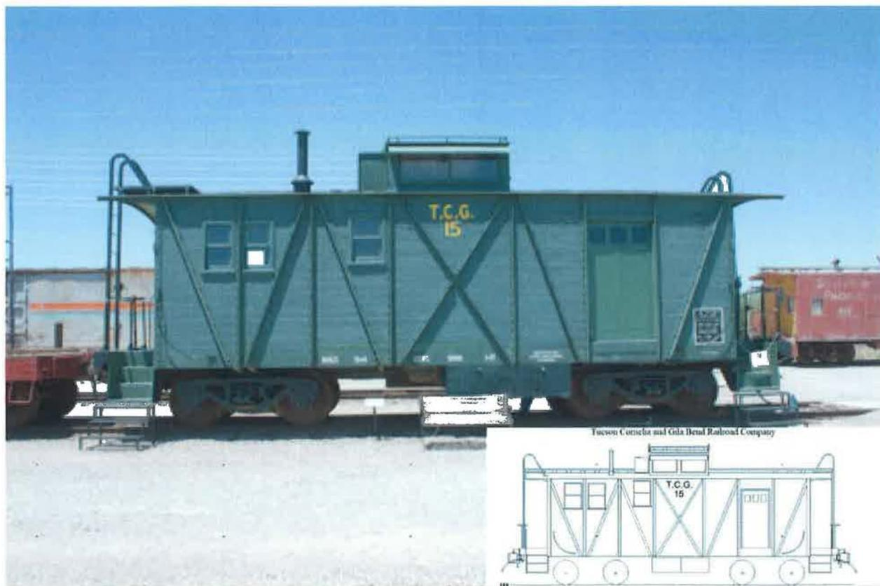
Figure 4. The TCG 15's distinctive three-part interior division is expressed on the exterior with, in the passenger seating area (left), a pair of double-hung wood windows and one double-hung wood window at the restroom location; central access to the cupola; and the rear cargo area. Photo source: A. Reigelsberger, 2016; inset schematic: T. Klobas, 2017.
