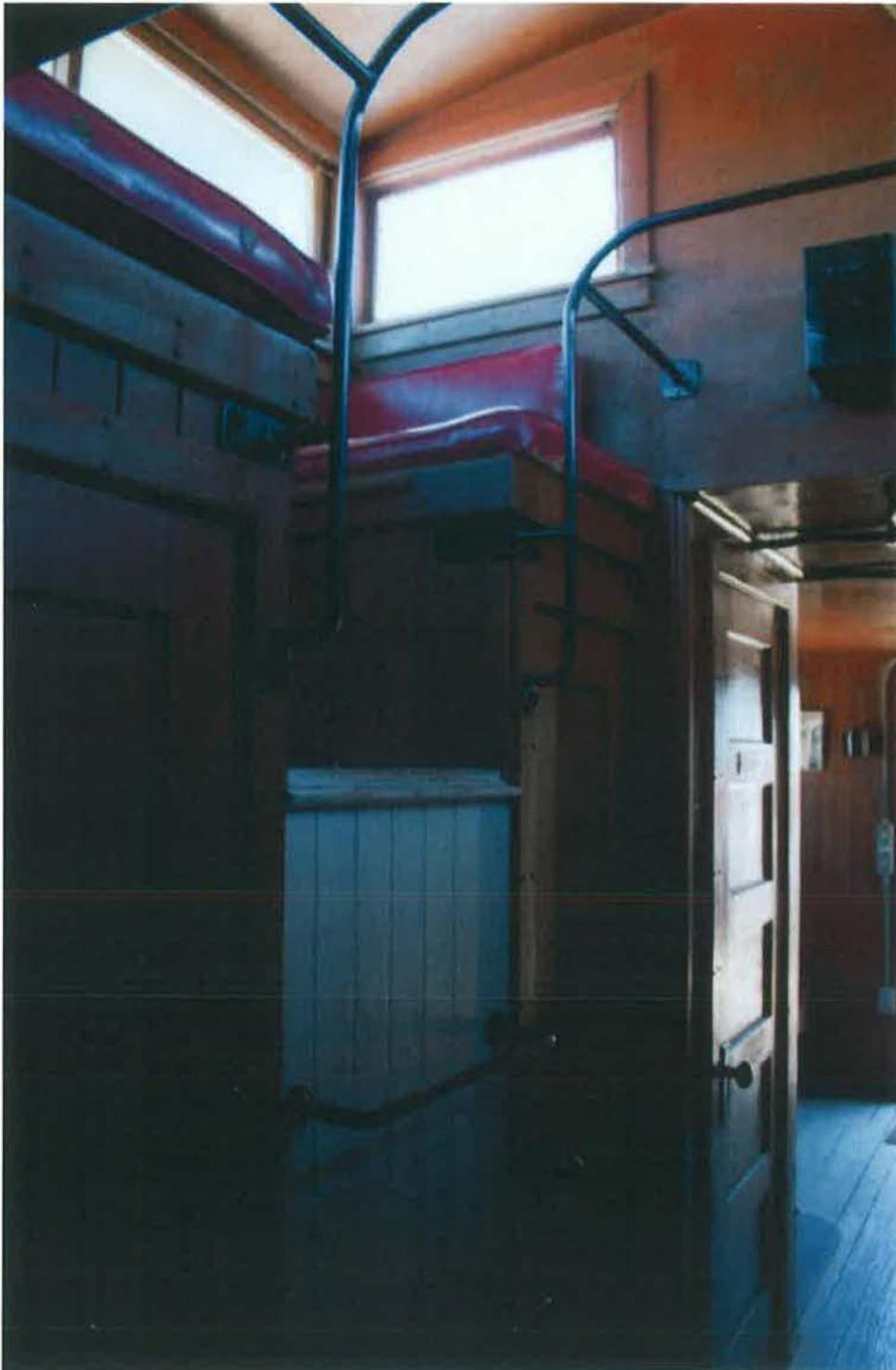
AZ\_Maricopa County\_TCGB Caboose #15\_0008. Interior of caboose center section showing cupola seating, access ladder, storage areas, restroom entrance, and passageway to passenger section
