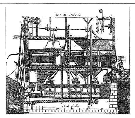
Fig. 4 Ollver Evans' Automatic Mill of 1791. This picture has often been reproduced, but only in his own "Young Millwright and Millers' Guide" is the complete description given. The leading features are: 1-Wagons emptying grain into scale pan. 2-Scale pan to weigh the grain. 3-Small garner and wind chest for cleaning wheat. 4. 5-Elevator to top floor of mill. 6-Main store for wheat. 7-Garner feeding the shelling or rubbing stones.
