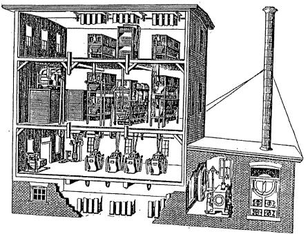
Fig. 8 Cutaway view of an 1892-roller system flour mill. This represents one of the Edward P. Allis Co.'s latest fifty-barrel flouring mill, the building being 30x40 ft., with basement and three stories. The mill house is of frame and the engine room is of brick. Note the increased height of the second story. (From their catalogue "Small Modern Mills" as reprinted in <u>United States Miller</u>, (Dec. 1892), 271).
