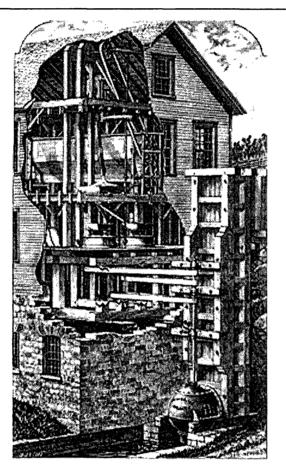
Fig. 3 Superior efficiency, all-season usefulness, and low cost led the American mixed-flow type turbine (which channeled water inward and then downward) to displace the traditional overshot wheel and others. Illustrated here is the method of transmitting power from the turbine to run two millstones. ("Leffel Turbine Wheel Driving a Two-Run Flouring Mill," *United States Miller*, 16(January 1884), 37)
