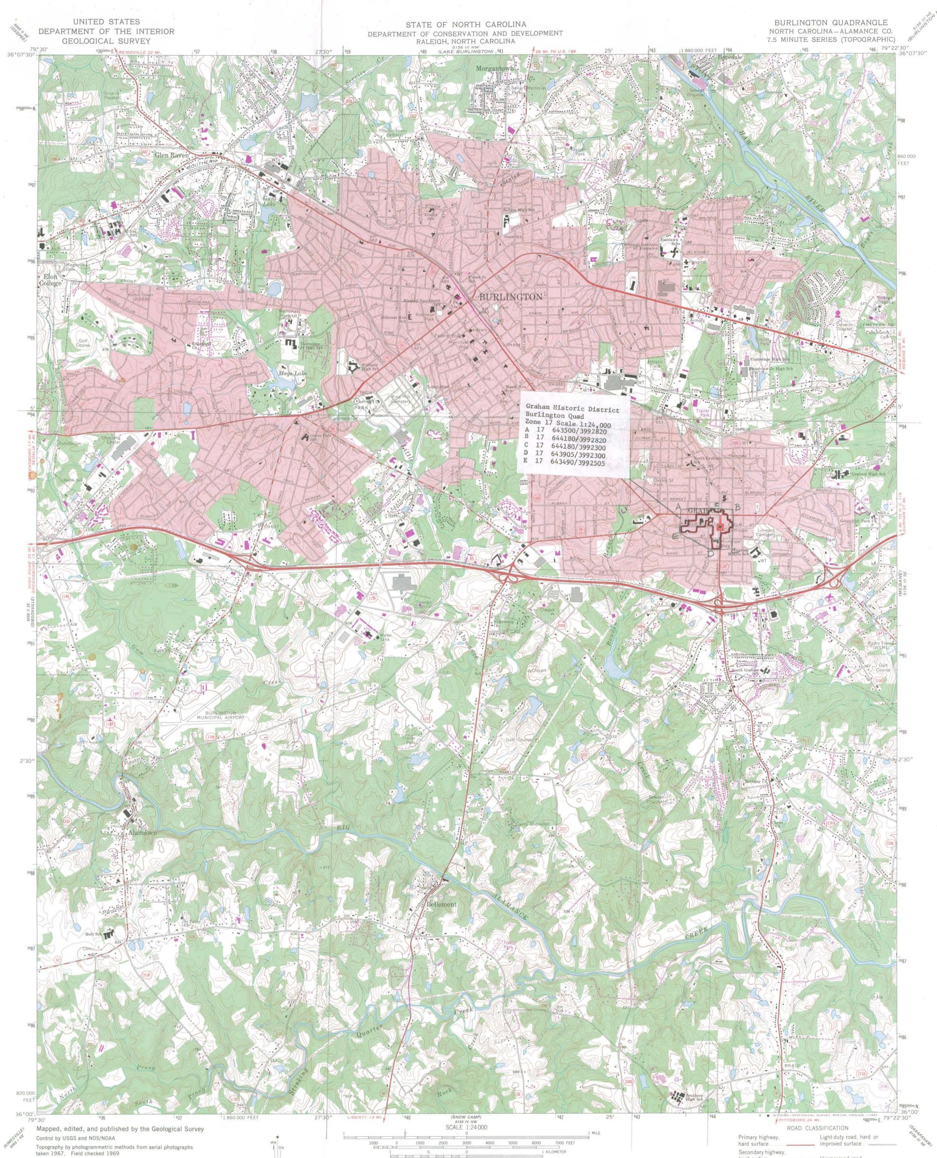
Polyconic projection. 10,000-foot grid ticks based on North Carolina coordinate system. 1000-meter Universal Transverse Mercator grid ticks, zone 17, shown in blue. 1927 North American Datum To place on the predicted North American Datum 1983 move the projection lines 11 meters south and 21 meters west as shown by dashed corner ticks
